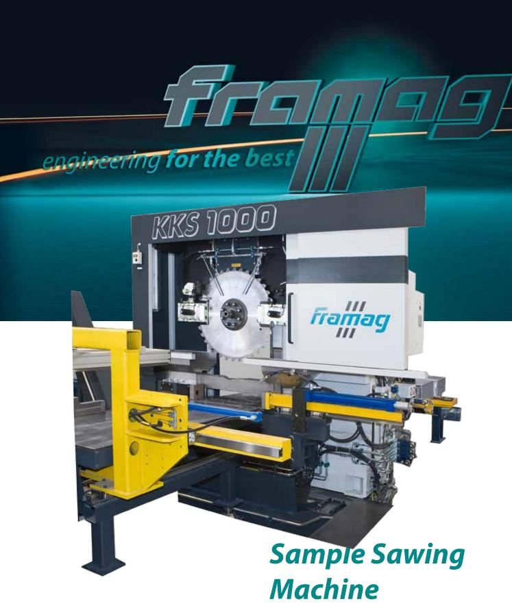
**framag's SAMPLE SAWING Machine** has been developed for high efficiency cutting of steel samples, where high reliability is required. Carbide tipped saw blades are used, enabling to cut with high efficiency without coolant water, to reduce production costs and to save the environment.
